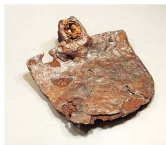
fig-17: Rusting of iron
